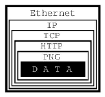
In this example, we are trying to get an image from a web page we are connected to via an Ethernet.
