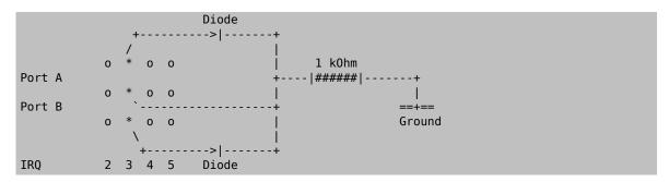
The cathodes of the diodes are connected to a common point, together with a 1 kOhm pull-down resistor. It is essential to connect the resistor to ground to avoid floating of the IRQ line on the bus.
